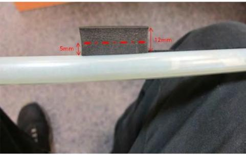
$2. \ Remove the felt strips from the locations highlighted on the roller blind assembly$
