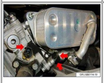
Example: A-Three Heat Exchanger **Light external engine oil accumulation No repair is necessary.**
