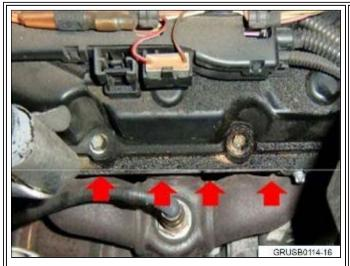
Example: B-One Cylinder Head Cover Gasket **Medium to large external engine oil accumulation**
