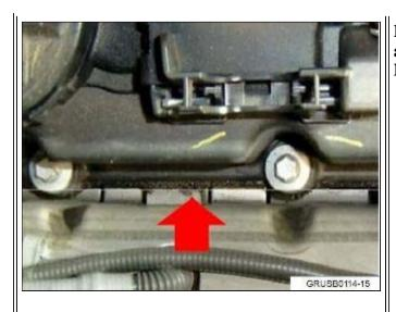
Light external engine oil accumulation No repair is necessary.
