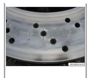
1. Visible cracks are caused by high thermal stresses during rapid heating and cooling of the brake discs. Braking from high speed with cold brake components (less than 212 degrees F) increases the likelihood of cracks to form. These surface hairline cracks are usually spread over the entire brake disc friction area, and have no negative influence on the durability or braking performance. The rotors should not be replaced only for their appearance reasons.
