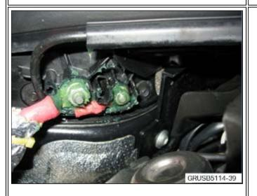
• Coat the battery positive terminals in the engine compartment with contact grease, using a locally sourced flat brush.
