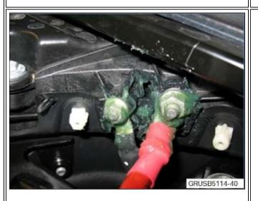
• Coat the battery positive terminals in the engine units compartment with contact grease, using a locally sourced flat brush.
