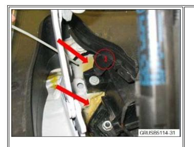
• Thoroughly spray cavity wax to the bulkhead in the area of the dynamic strut, in the areas shown in the picture.
