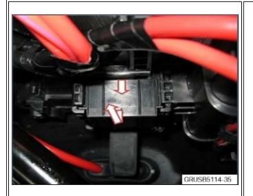
• Remove the cover on the battery positive terminal in the direction of the arrow, and replace it.
