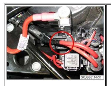
• This picture shows the installation location of the cover to be replaced, below the battery positive cable.
