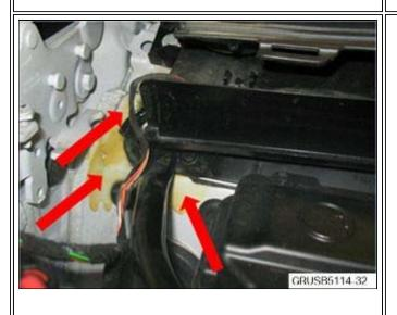
• The wax should be visible in the following areas after spraying.
