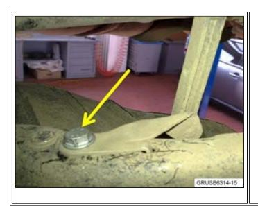
2. New If the hex bolt is broken, remove the broken bolt. (Unscrew the broken bolt out or, if necessary, drill it out.)
