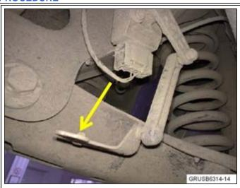
1. New Inspect the rear height sensor, located in the left rear of the vehicle as shown. If the sensor bracket is hanging loose, the hex mounting bolt has broken.
