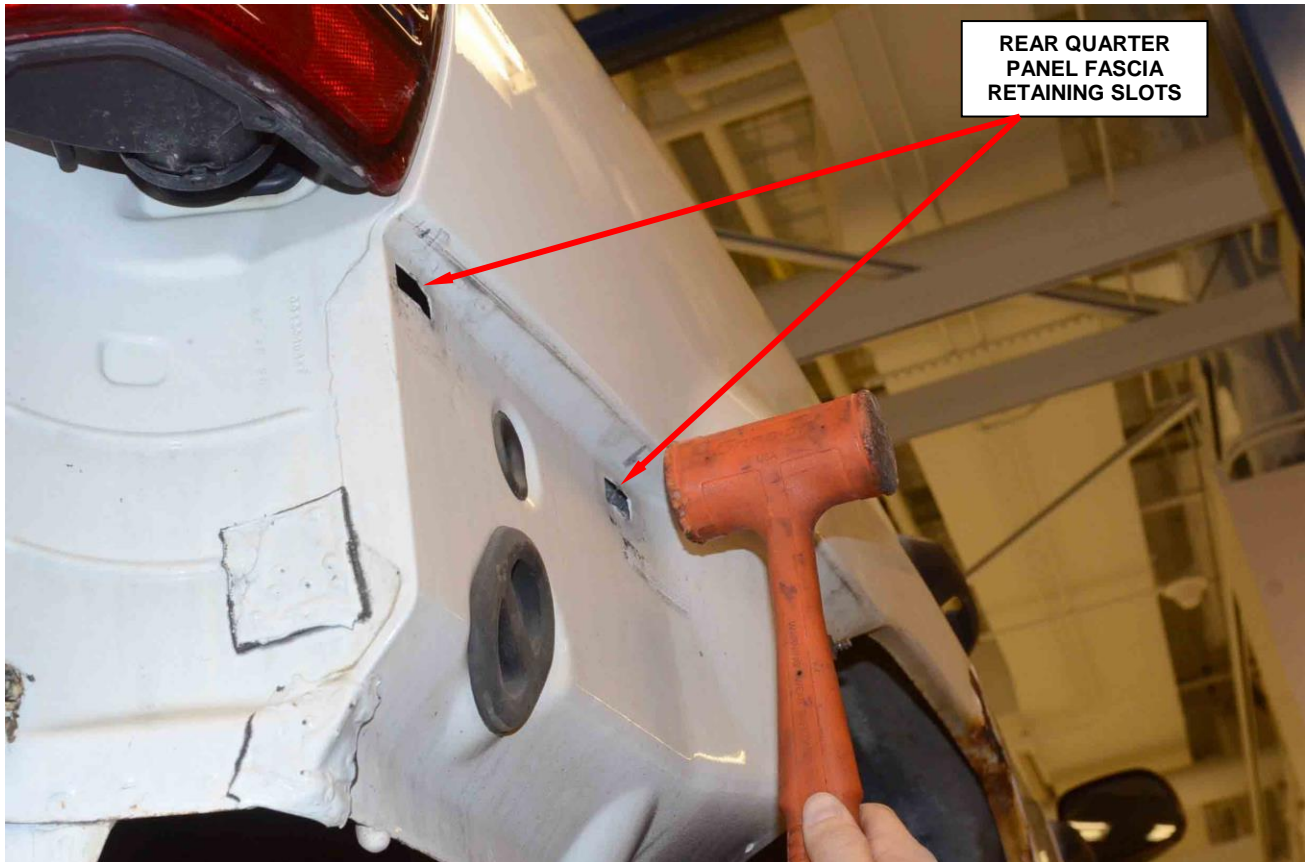
Figure 10 – Flatten Fascia Retaining Body Slots
