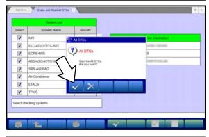
c. A window will pop up asking you to confirm DTC erasing. Click the check mark in the dialog box for DTC erasing and reading to begin.
