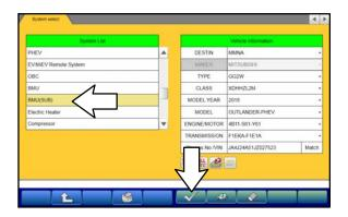
a. Select "**BMU(SUB)**" from the System List, then click on the check mark at the bottom of the screen.
