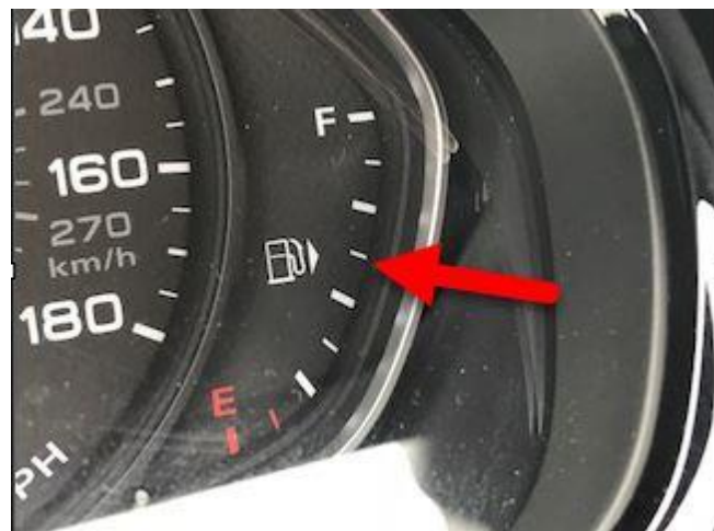
Figure 1. Only shows 5/8ths of a tank instead of full.
