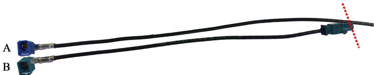
Figure 2. Measure the cut point on the vehicle's antenna coaxial wiring (A) based off the length of the replacement coaxial "Adapter Antenna Cable" (B). The removed length of cable from A should be equal to the length of cable B.
