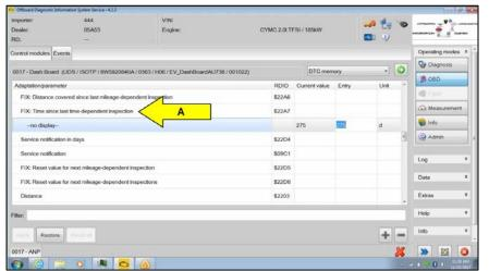
Repeat the above procedure with the same calculated value for the adaption value "FIX: Time since last time-dependent inspection" <arrow A>.
