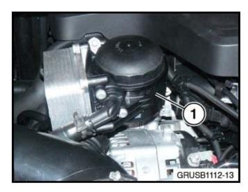
Vehicles produced prior to 6/2012 will be equipped with a black plastic oil filter housing (1). In this case, engine oil filter kit P/N 11 42 7 634 291 should be used.
