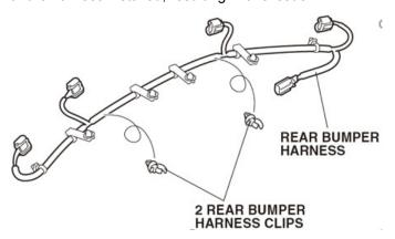
If any of the sensor retainers have separated from the bumper, order replacement retainers (P/N 08V67-TZ5-2M001). When installing them, be sure to thoroughly clean the rear bumper with isopropyl alcohol and a clean shop towel where the adhesive will attach.
