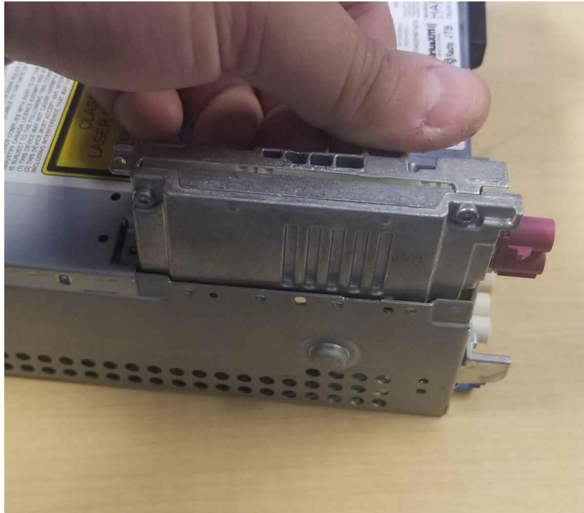
Figure 8. Do not press down using the purple FAKRA connector.
