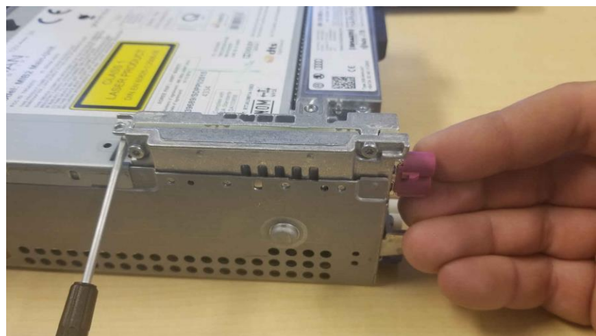
Figure 7. Lift up on both ends of the telephone module.
