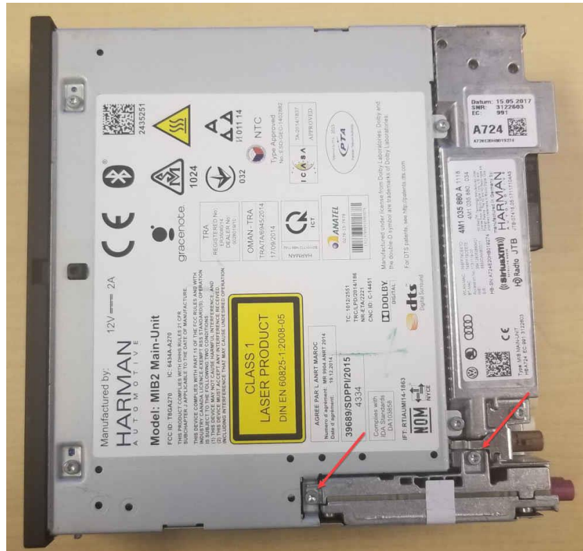
Figure 6. Telephone module retaining screws indicated by the red arrow.
