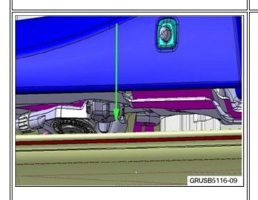
4. Place the spray lube nozzle at the upper end of the rail for the window guide. Use a good amount of spray lube in this area.
