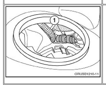
4. Inspect the fuel hose (1) for splitting. It might be necessary to inspect the entire circumference of the fuel hose with a small mirror. If the fuel hose (1) is found to be split, replace the fuel tank. Do not attempt to replace or re-secure the fuel hose inside the fuel tank.
