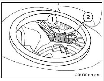
3. Inspect the fuel hose connection (1) on the pressure regulator (2). If the fuel hose is found to be disconnected from the fuel pressure regulator, replace the fuel tank. Do not attempt to replace or re-secure the fuel hose inside the fuel tank.
