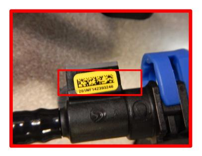
Correct and Suspect parts can be identified by the color of the label on the sensor.
