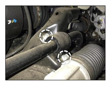
7. With the four (4) steering gear assembly mounting bolts removed, place a 2x4 block of wood underneath the steering gear assembly for stability of the assembly during this repair procedure.
