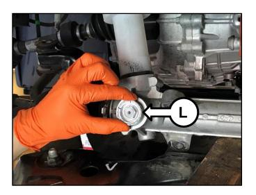
18. Tighten and torque the yoke plug (L) to specifications.
