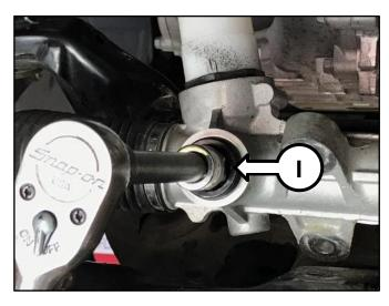
10. Remove the yoke spring (J) and set aside for reinstallation.
