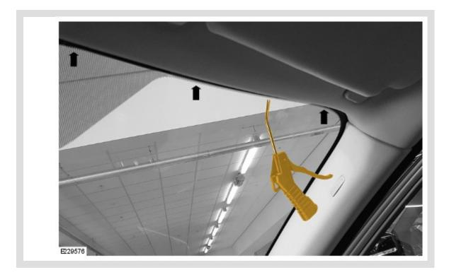
Use an air blower to blow compressed air around the edge of the inner side of the windshield as shown.
