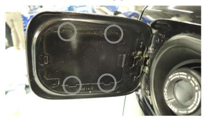
4. Installation of the new fuel filler lid is the reverse of removal. Verify all the tabs are engaged, and slide the lid away from the fuel fill door hinge until it clicks. This indicates the fuel filler lid cover is secured and correctly installed.
