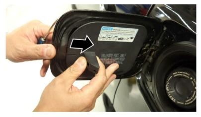
3.3. Slide the lid until the four tabs disengage from the slots in the fuel fill door.
