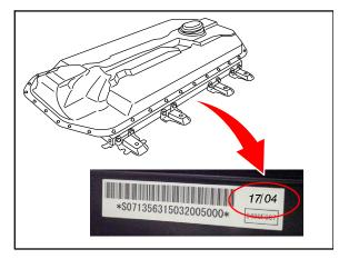
Locate the label on the drive battery, and find the production date in upper right corner.
