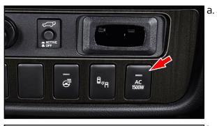
To enable power to the 120V AC outlets on the Outlander PHEV, press the "AC 1500W" switch in the front instrument panel (below the A/C controls).
