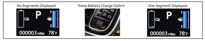
• If one or more segments are displayed, press the POWER button to enable "READY" mode and maintain for 30 minutes. This will charge the 12V auxiliary battery.
