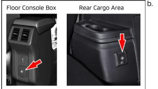
Verify the outlet(s) function properly when an electrical appliance (e.g., coffee maker, blender, etc.) is connected.
