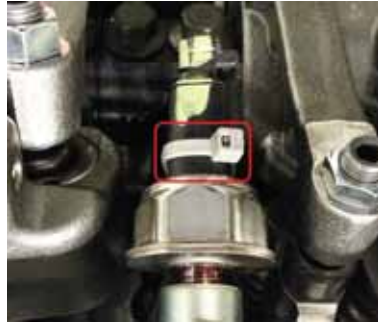
Cable tie location
