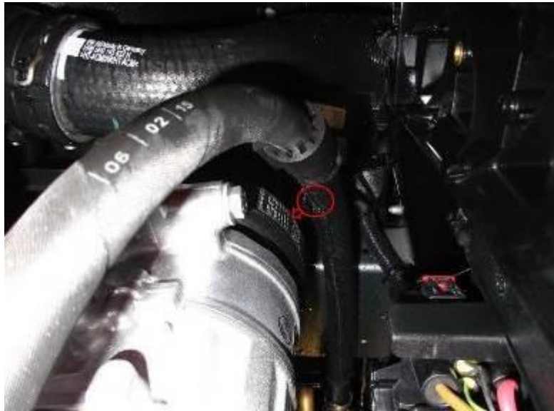
Figure 2. Point of hose contact with air conditioning compressor pulley – rear view.
