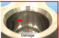
Foreign Material – **OK Part** Compressor has foreign material stuck to seal bore.
