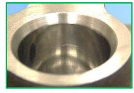
Damage – **No Good Part**Compressor seal bore is damaged due to deep scratching perpendicular to O-ring groove.
