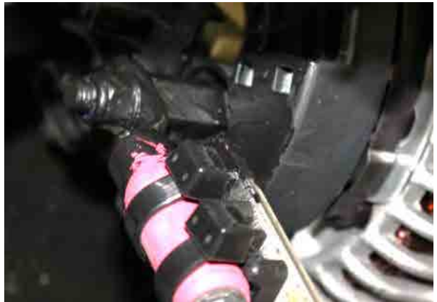
FIGURE 80: POSITIVE (+) CONNECTION ON THE ALTERNATOR
