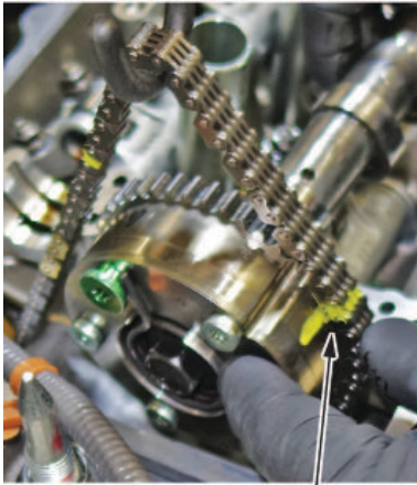
As the camshaft is installed, line up the marks made in step 3.
