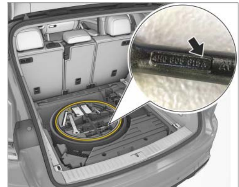
Tool kit with towing lug (with collapsible spare wheel)
