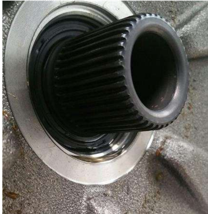
Figure 2. Oil leak at the input shaft.
