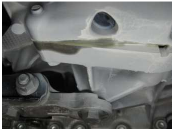
Figure 1. Oil leaking from the bellhousing.
