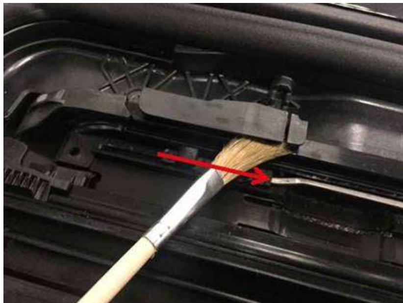
Figure 5. How to apply grease.
