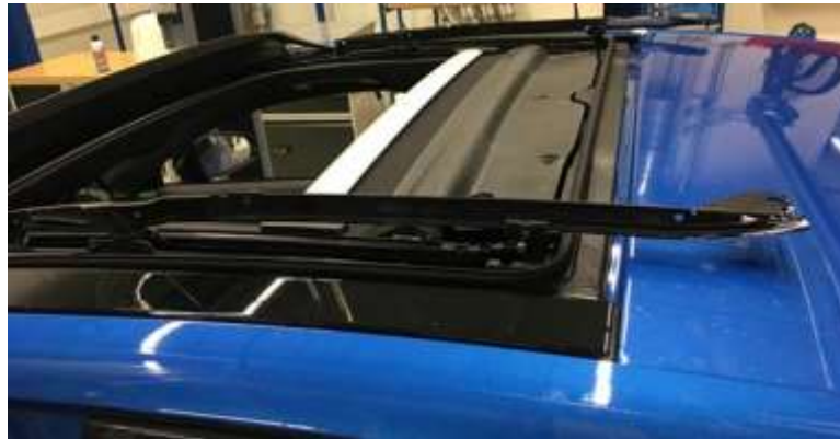
Figure 1. Sliding rails exposed showing the area of contamination.
