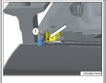
5. Using the access hole from step 2, spray cavity protection spray PN 83 42 2 457 337 between the inner door hinge support and the door.
