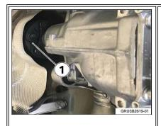
Raise the vehicle to inspect the flex disc at the rear differential (1).
