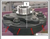
A flex disc installed incorrectly will have the burr closer to the rear differential (1).
