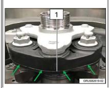
A properly installed flex disc will have the burr closer to the front of the vehicle (1).
