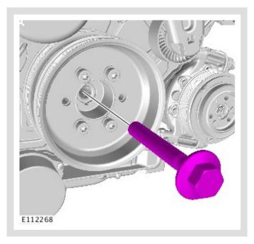
Remove and discard the center main crankshaft pulley bolt(s).
