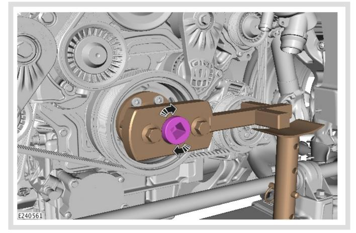
Remove the from center main crankshaft pulley bolt(s).
