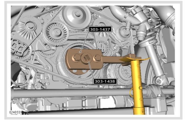
Use a suitable vehicle stand to support the special tools 303-1437 and 303-1438.
