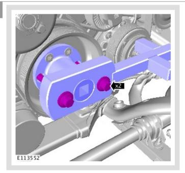
Remove the 2 bolt(s) from special tool 303-1437.
