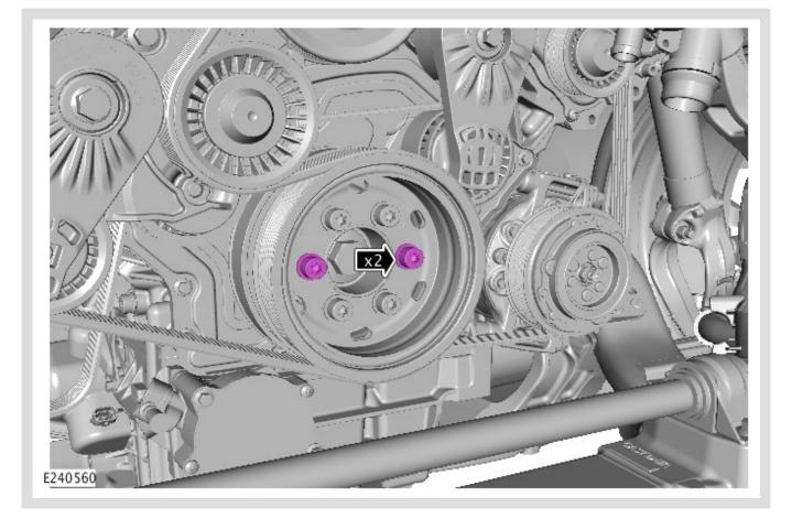
Remove and set to the side only the 2 highlighted outer crankshaft pulley bolt(s).
