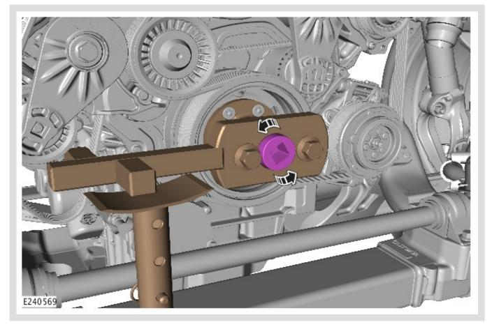
Tighten the center main crankshaft pulley bolt(s) in 2 stages. Make sure that the socket is turned through 270°, not the torque wrench.
