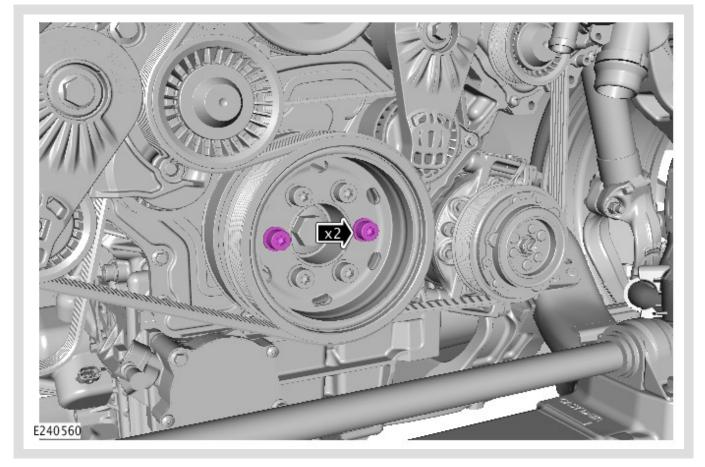
Install the original outer crankshaft pulley bolt(s).
