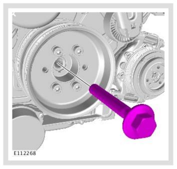
Install the new center main crankshaft pulley bolt(s).
