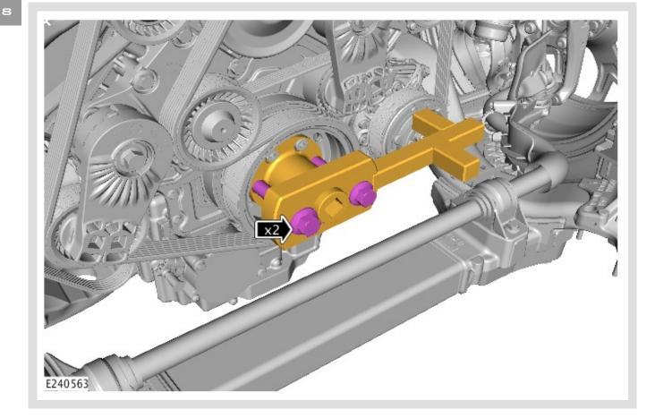
Remove the 2 outer crankshaft pulley bolt(s) from special tool **303-1437**.
