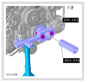
Remove the vehicle stand and special tools **303-1437** and **303-1438**.
