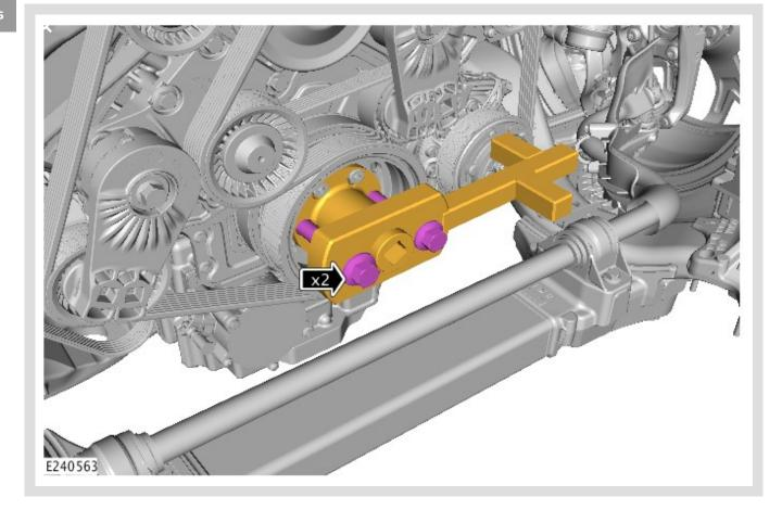
Using the bolt(s) for special tool 303-1437, install the 2 bolt(s) to the crankshaft pulley.
