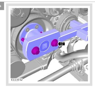
Using the bolt(s) for special tool 303-1437, install the 2 bolt(s) to the crankshaft pulley.
