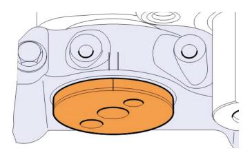
**2.** Once the timing marks are aligned for a specific Injector Pump, verify the injector rocker roller is on the base circle of the injector lobe. Refer to the illustration below.
