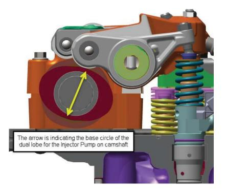
**Note:** If an injector lobe rotates on the camshaft, the rotation is normally by 60 degrees. It takes approximately 15 degrees of rotation before potentially causing the faults codes listed previously or a fault for a pumping injector during the Common Rail Fuel System Test.
