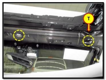
4. Apply the Loctite to the front sunroof mounting bolts (U).
