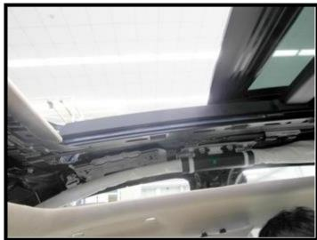
9. Remove the mounting bolts (X) on the moveable glass.
