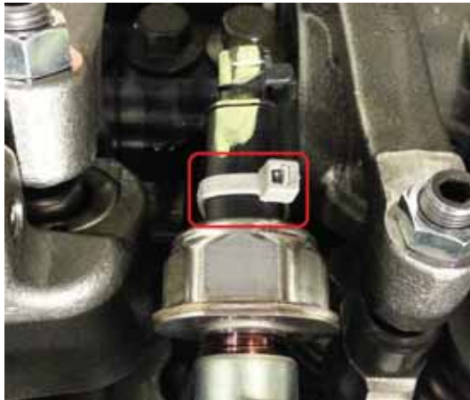
Cable tie location
