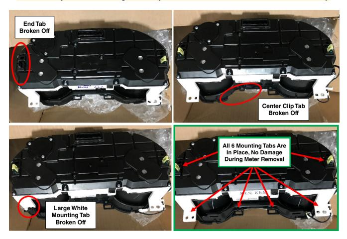
**Step 6: NOTE:** Previously, the removal procedure showed releasing the top claws on each end then grasping the bezel with the thumb and forefinger and pulling straight back to release the 2 center retaining clips.
