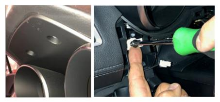
**Step 9:** Cover the steering column cover with a clean cloth or towel to protect it while removing and reinstalling the combination meter. **CAREFULLY** pull the meter toward you enough to get a hand behind it. Press the lock tab on the wiring harness connector and unplug it. There is only the one connector. Once unplugged, remove the combination meter from the IP toward the right of the steering wheel.
