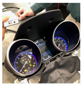
While the update is happening, the Yellow LED will blink on and off. When the update is complete, both the Green and Yellow LEDs will both come on solid. At this point, should the Red LED come on, repeat this (Step 10) again from the beginning. After successful completion, unplug the tool harness from the combination meter and the power supply from the wall outlet. This "resets" the tool.
