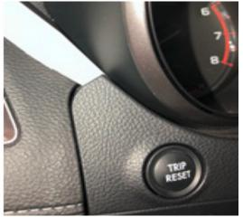
• Release the lower claws on both ends of the bezel using a trim clip removal tool as shown. When all four corners are released, the bezel will appear loose as shown in **Figure 1** below **BUT**, there are 2 more upper / center retaining clips which must be **CAREFULLY** released from underneath before the bezel can be removed.
