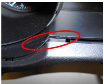
Use the photos below for reference when **CAREFULLY** removing the combination meter lower trim bezel.
