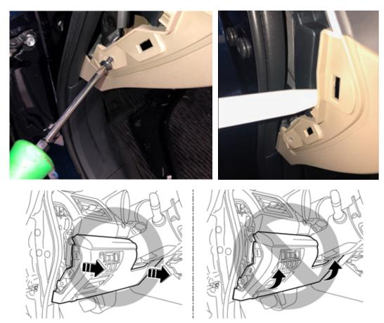
**REMINDER:** Before proceeding to **Step 6** below, it cannot be stressed enough for Technicians to **TAKE THEIR TIME** when removing and reinstalling the combination meter. The photos below illustrate what can happen to the meter assembly when not performing these steps **CAREFULLY**. These 3 examples all show damage caused by outside influence which is not a matter for warranty.
