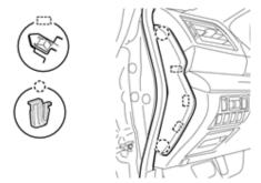
**Step 5:** Remove the philipps screw and release the 1 clip on the end portion of the trim shown in the photo. Then, **CAREFULLY** release and lower the lower IP trim panel by pulling it straight back toward you. **DO NOT** try to "peel" it up from the bottom. Leave all switches and the aspirator tube connected. Support the lower IP trim so there is no tension on the switch connections or harnesses.
