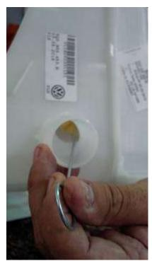
Figure 4. Cleaning the sensor probes.
