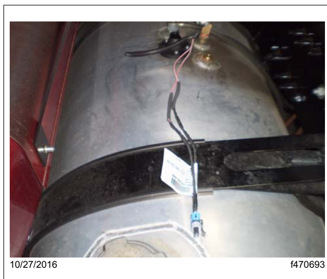
Fig. 9, New Pigtail Installation
