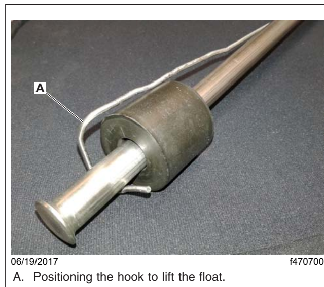
Fig. 5, Lifting the Float
