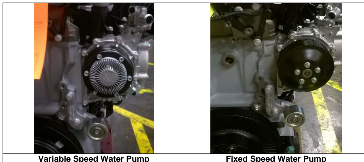
Figure 1 – Water Pump Identification
