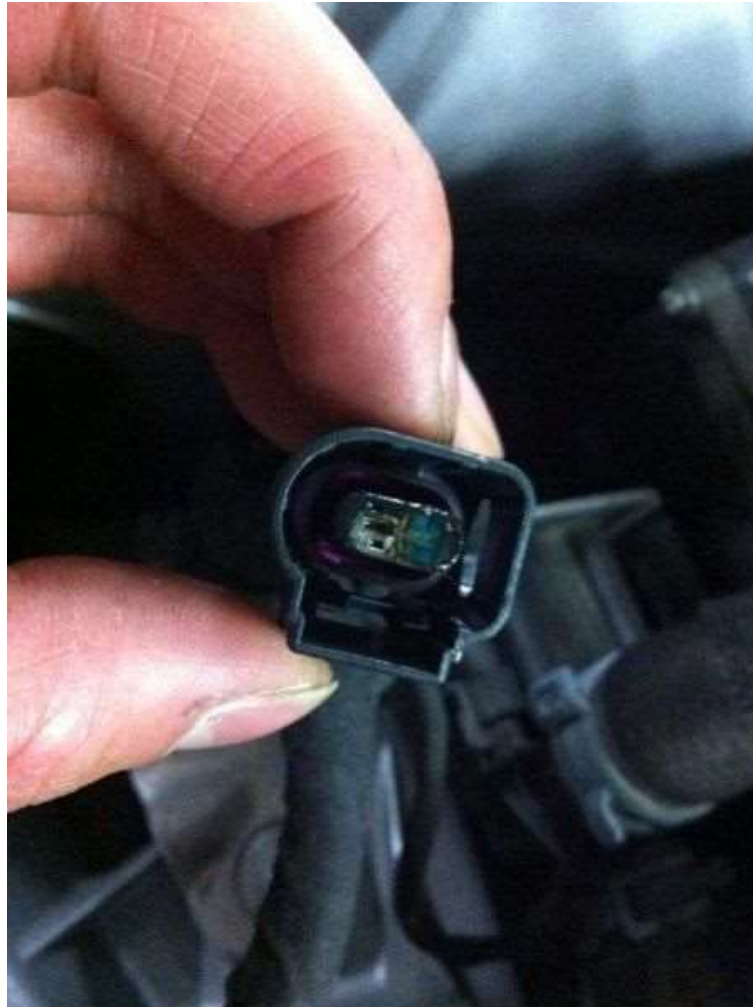
Figure 2. Corrosion formation on the connector pins.
