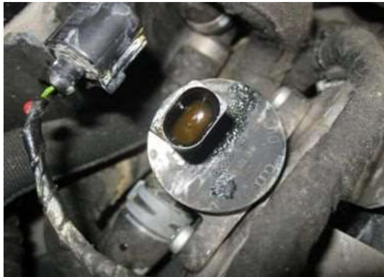
Figure 1. Coolant residue in the connector housing of the coolant regulating valve.
