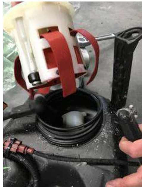
Figure 1. Filter element housing loose inside tank.
