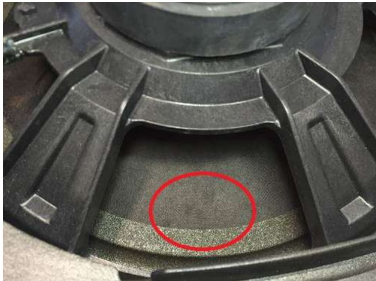
Figure 1. Deformation of the speaker cone.
