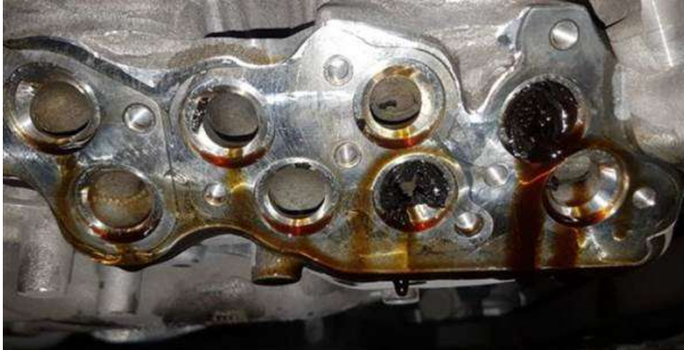
Figure 1. Example of closed oil drains on oil baffle plate.
