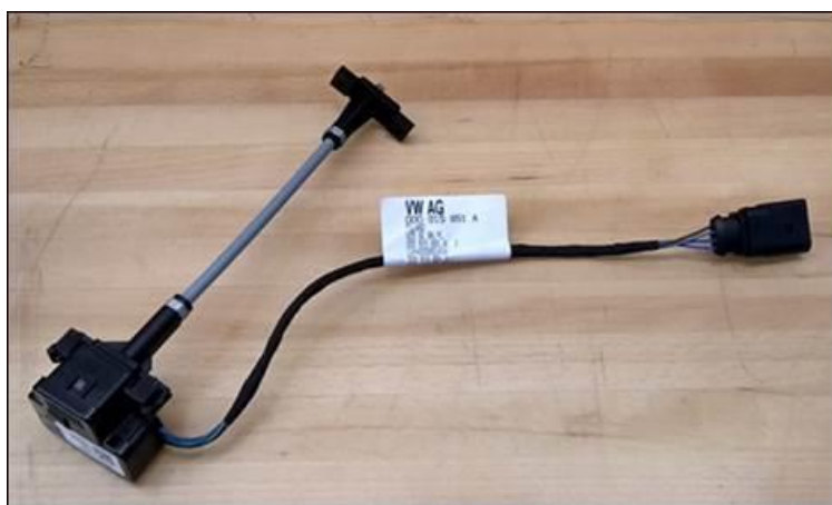
Figure 1: Repair kit actuator -F498- for North America (for use with NAR-version AC/DC Combo Socket).
