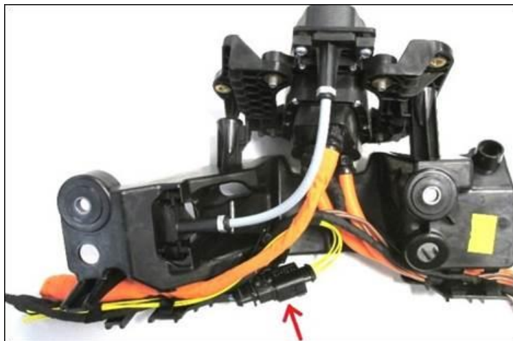
Figure 2: Finished location of new connector and correct wire routing. Repair wires (in yellow) are shown without tape for clarity only. The splices and wires must be properly wrapped in cloth tape part number N 10592002 for protection in actual repair.
