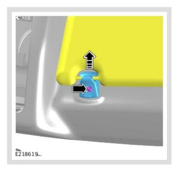
Release the sun visor, remove the bolt(s), and remove the clip.
