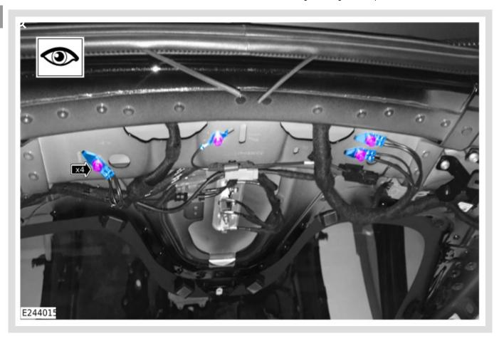
Locate the 4 ground points, remove the 4 bolt(s), and reposition the eyelets.
