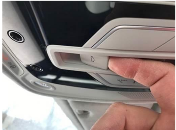
Figure 1. Set the sunroof panel basic settings by pulling the sunroof switch fully downward.
