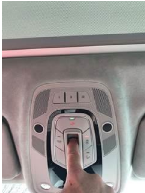
Figure 2. Set the sunroof shade basic settings by pushing the sunroof shade switch fully forward.
