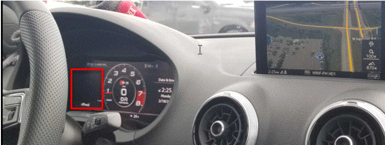
Figure 1. Map section is blank in the instrument cluster display.
