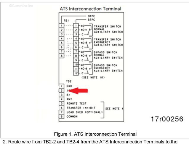
2. Route wire from TB2-2 and TB2-4 from the ATS Interconnection Terminals to the external Remote Start connection terminals found on the Rental generator set control box panel.
