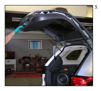
Open and close the tailgate a few times to verify there is no noise generating from the gas springs when opening and closing the tailgate.
