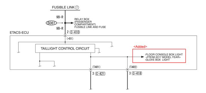
Please make the indicated changes below to the 2014 - 2019 Outlander Service Manual, Group 90-Circuit Diagrams, "Glove Box Light and Floor Console Box Light" diagram.
