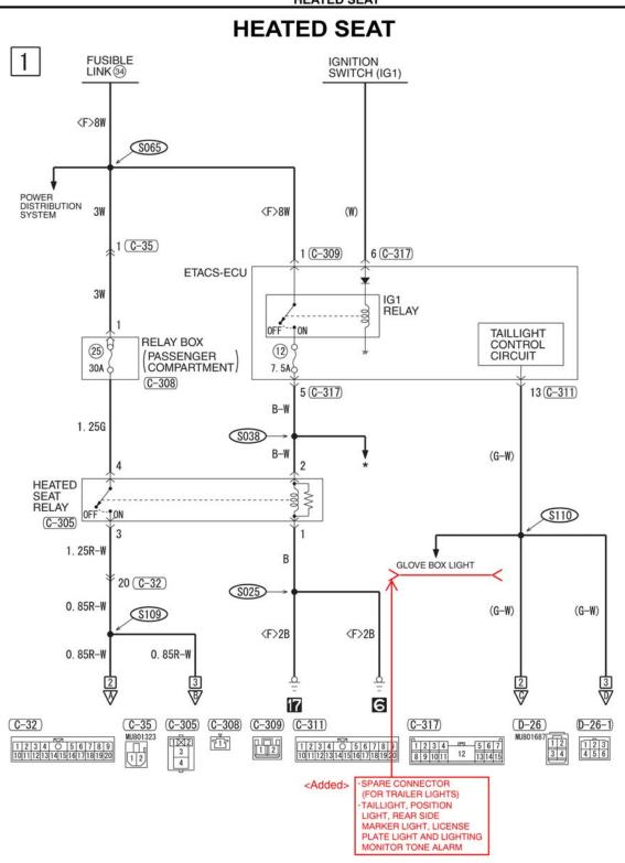
Please make the indicated changes below to the 2014 - 2019 Outlander Service Manual, Group 90-Circuit Diagrams, "Taillight, Position Light, Rear Side Marker Light, License Plate Light and Light Reminder Tone Alarm" diagram.
