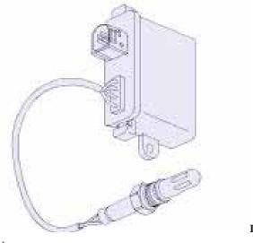
Installation torque of 50 Nm +/- 5
